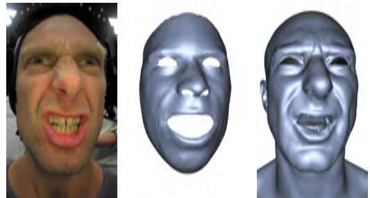
Figure 14: Left: An input frame. Middle: Real-time monocular method of Thies et al. Right: Our real-time method using 2 cameras.
