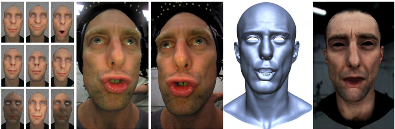
Figure 1: We propose a real-time multi-view face tracking method for high-quality on-set facial performance capture. Using rendered synthetic training (left most) we learn an actor-specific regression function, which tracks the actor's face online using multiple cameras (middle left). An reconstructed expression is depicted (middle right) together a digital-double face rig within a game engine (right).
