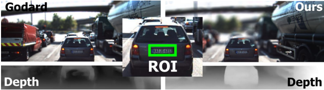
Figure 9: Experiments on real data. The region of interest is set with 2D tracking onto the number plate (middle) and the corresponding depth value is recovered. The left illustrates refocusing using a depth map generated by [14] while we show on the right the result of our sequential refocusing pipeline, together with the underlying disparity map.
